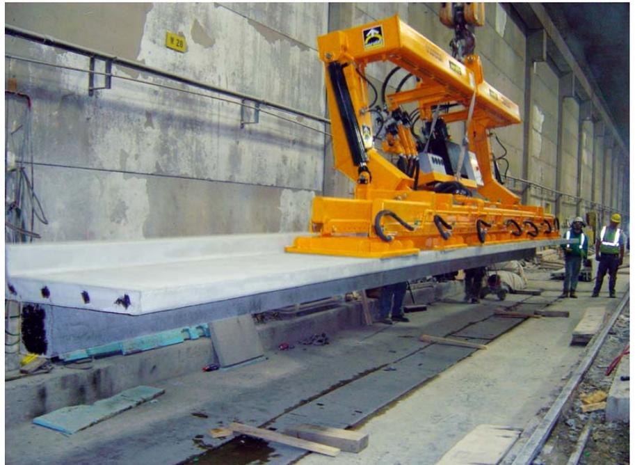
*Aerolift handling device inside the Hanson production factory, de-moulding and 90 degrees turning*
